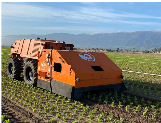
FarmWise Titan, a semi-autonomous weeding robot (Photo: FarmWise)
